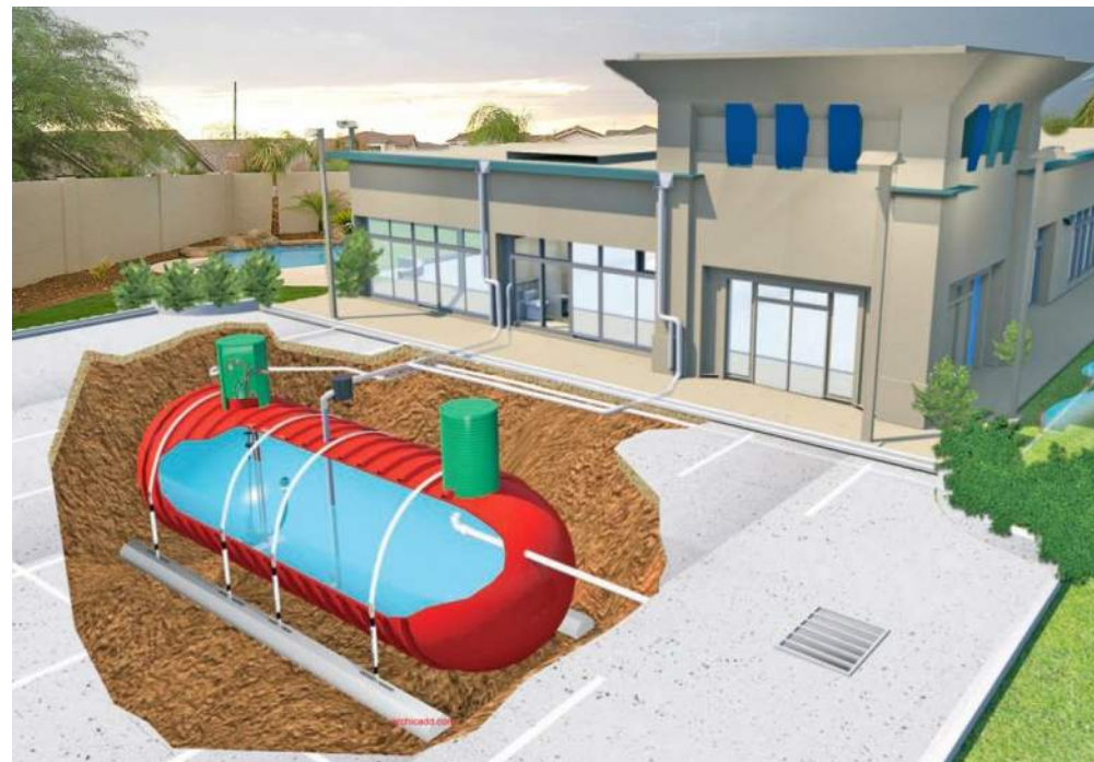
Figure 9.5 – Indicative Rainwater Harvesting Layout
